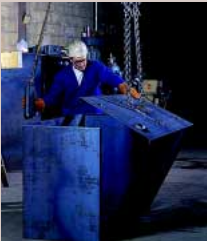
Single-wall UL-142 Lube Tank Mild carbon steel meeting ASTM specifications is used in all tank construction. Stainless steel can be specified.
