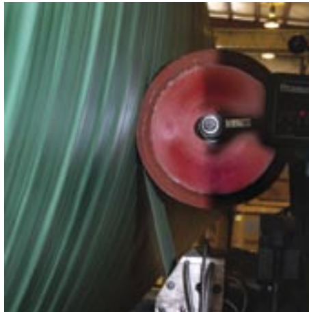
The secondary containment tank wall of High Molecular Weight Polymer is extruded and applied hot, under pressure.
