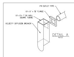
NOTE: BUDYANCY RESTRAINT NOT SHOWN CUSTOMER TO ADDRESS BEFORE INSTALLATION CONTACT HIGHLAND TANK FOR OPTIONS
