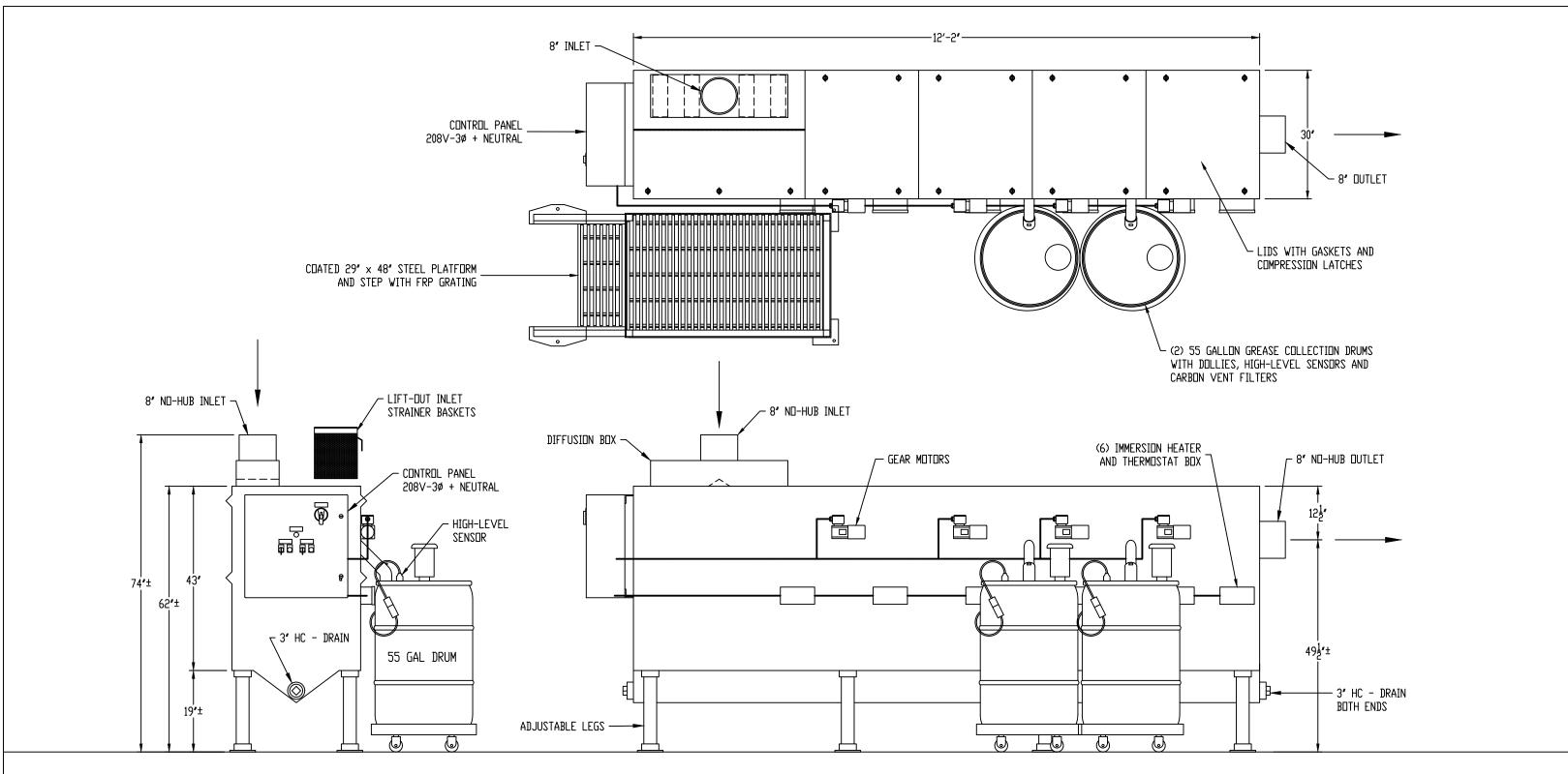
STANDARD CONTROL PANEL OPERATES ON 208V-3Ø + NEUTRAL SERVICE VOLTAGE - OPTIONAL PANELS AVAILABLE
