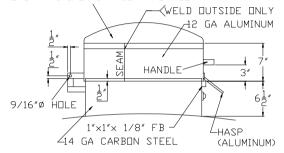
NOTE- DO NOT CUT HOLE IN HEAD FOR CHAMBER, WELD CHAMBER TO DUTER HEAD
