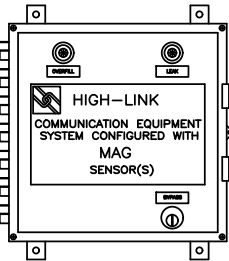
COMMUNICATION BOX DETAIL
