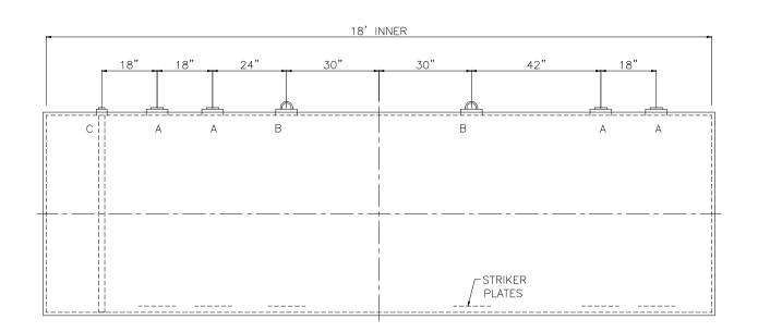
STRIKER PLATES ROLLED & SEAL WELDED TO THE TANK, 1/4" X 12" x 12" MIN.
