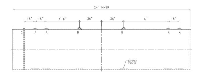
STRIKER PLATES ROLLED & SEAL WELDED TO THE TANK, 1/4" X 12" x 12" MIN.
