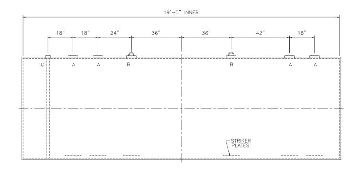
STRIKER PLATES ROLLED & SEAL WELDED TO THE TANK, 1/4" X 12" x 12" MIN.
