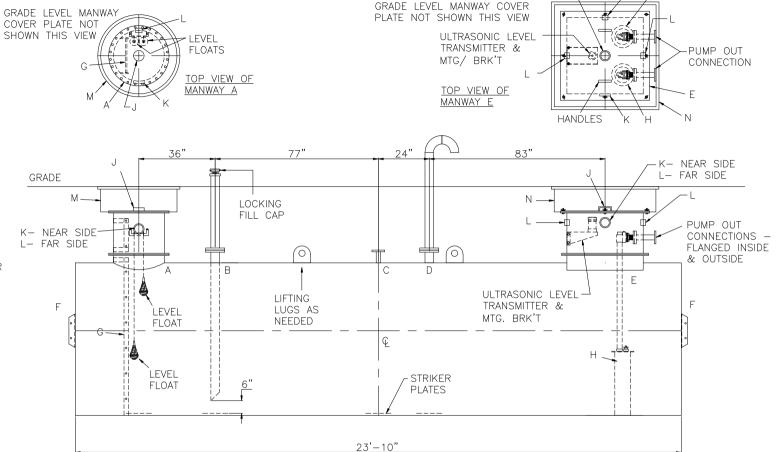
NOTE: AT LEAST ONE 2" VENT PIPE MUST BE INSTALLED IN EACH MANWAY RISER
