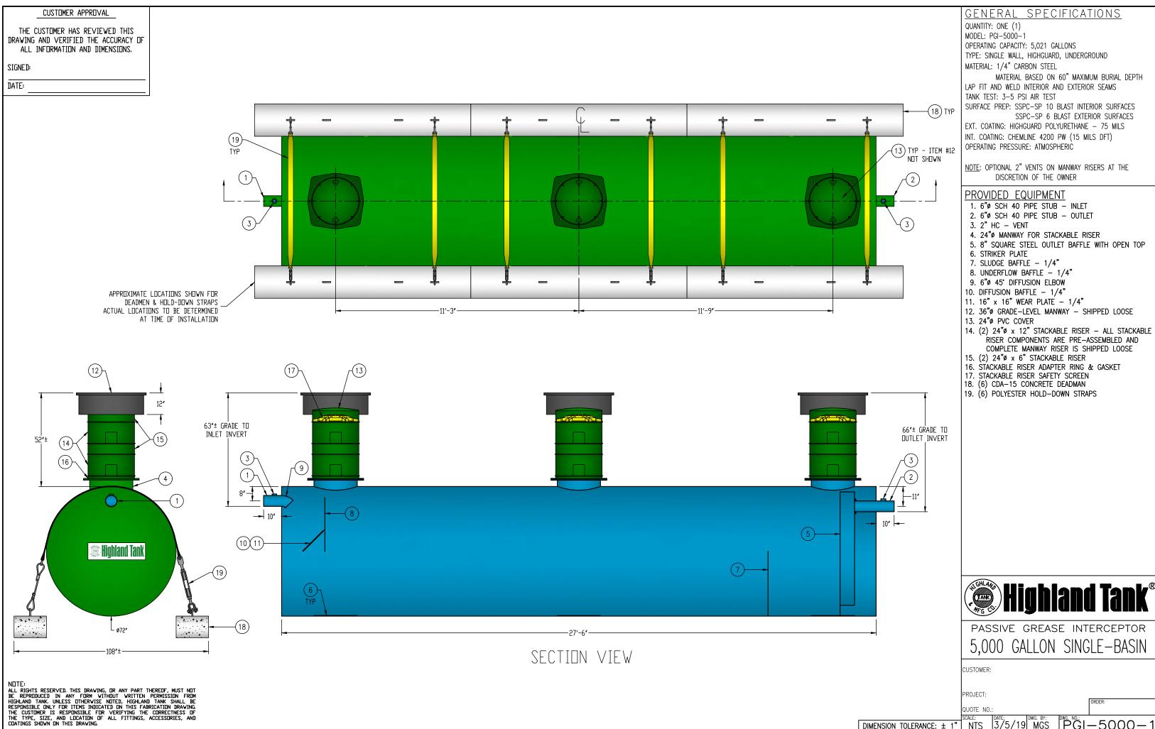
DIMENSION TOLERANCE: ± 1" SCALE: NTS 3/5/19 MGS PGI-5000-1
