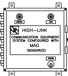
COMMUNICATION BOX DETAIL
