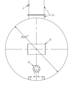
UNLESS NOTED, TOLERANCES ARE +/- 1 'HighDRO® WATER STORAGE TANK 8,000 GAL 96"Ø SINGLE-WALL UNDERGROUND HORIZONTAL FOR FIRE PROTECTION WITH BOTTOM DRAIN
