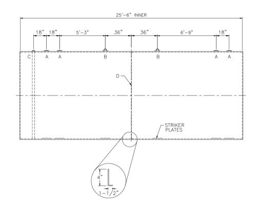
STRIKER PLATES ROLLED & SEAL WELDED TO THE TANK, 1/4" X 12" x 12" MIN.
