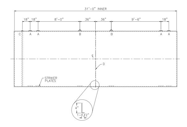
STRIKER PLATES ROLLED & SEAL WELDED TO THE TANK, 1/4" X 12" x 12" MIN.
