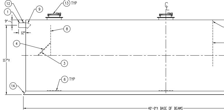
PROVIDED EQUIPMENT 1. 8"Ø SCH 40 PIPE STUB - INLET
