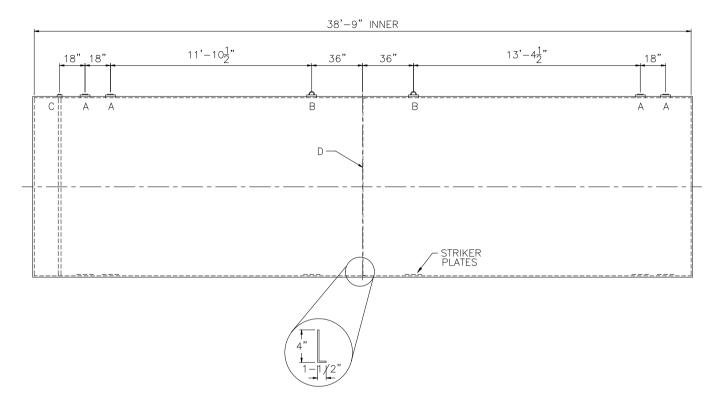
STRIKER PLATES ROLLED & SEAL WELDED TO THE TANK,  $1/4" \times 12" \times 12"$  MIN.
