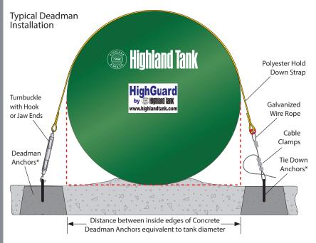
Top of deadman anchors level with bottom of tank. Fill area between deadmen with 12" or 18" approved bedding material\*.
