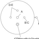
4" Fitting with 4x2 bushing, 2" pipe nipple and fill cap
