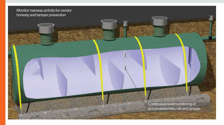
Highland Tank's passive grease interceptors are designed to remove large quantities of FOG discharged from food service facilities.
