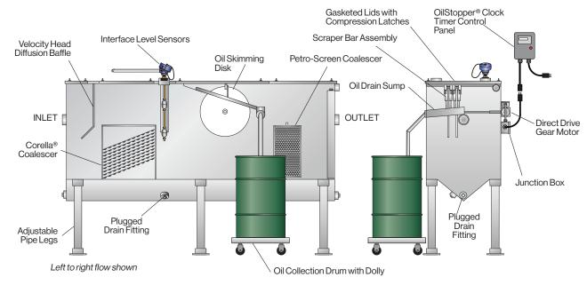
The Diskimmer helps reduce maintenance and waste oil charges by effectively only removing oil - not water. The OilStopper® operates at optimum efficiency by keeping the accumulated oil layer to a minimum.
