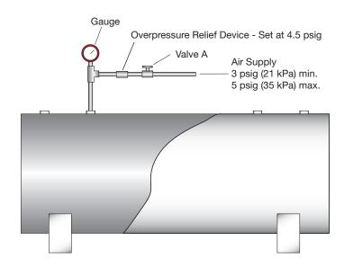
Fig 2. Vertical & Rectangular (non-Fireguard®) Single-wall Tank Air Pressure Test Set-up. Use calibrated diaphragm test gauge only with 0 to 3 psig on dial span.
