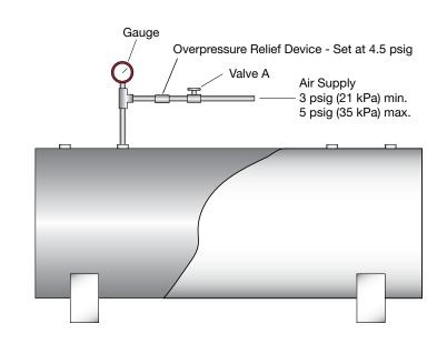
Fig 2. Vertical & Rectangular (non-Fireguard<sup>®</sup>) Single-wall Tank Air Pressure Test Set-up. Use calibrated diaphragm test gauge only with 0 to 3 psig on dial span.
