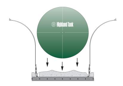
Position gap between angle plates as close to top center-line as possible. Secure the vessel in place by tightening nut at top center being careful to prevent vessel from turning or rolling from side to side.
