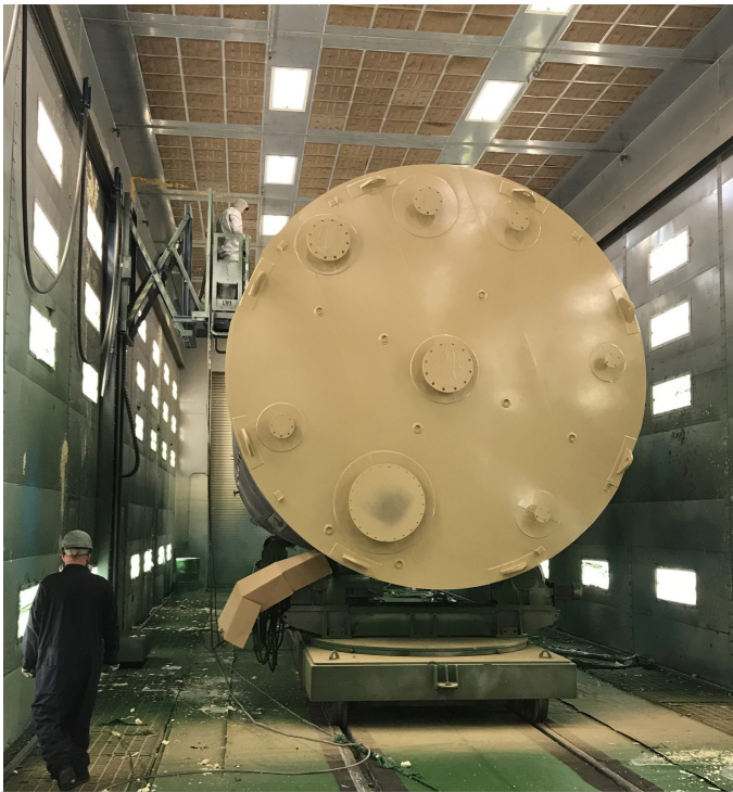
A vertical storage tank for renewable fuel oil in production.
