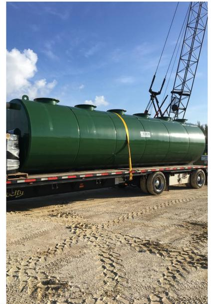
Universities and colleges serve many meals and generate huge amounts of grease. Highland Tank's grease interceptors help prevent that grease from causing an obstruction in the sewer line.
