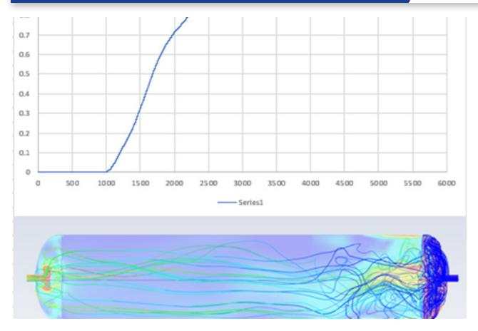
The inlet and outlet structures in the CCT are designed to distribute the water flow uniformly within the cross-sectional area of the contact chamber. Strategically positioned porous media within the contact chamber aid in achieving the minimum residence time requirements. The Highland Tank CCT hydraulic flow characteristics are proven to meet or exceed industry standards by providing an efficient engineered system to meet requirements of the EPA's Surface Water Treatment Rule.
