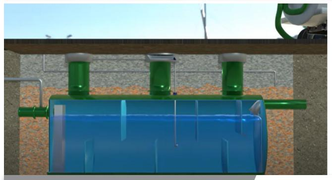
Check out our video on how the passive grease interceptor works to remove grease.
