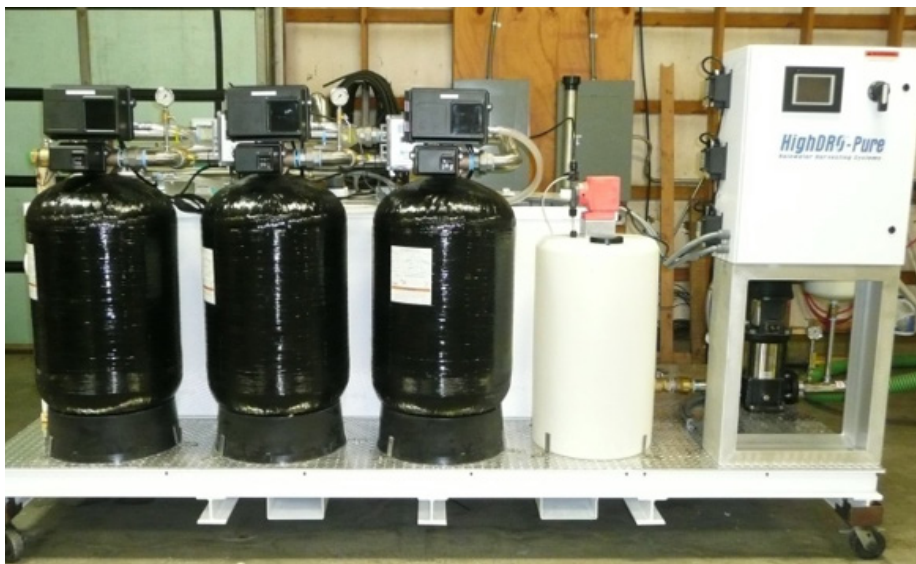
Rainwater Recycling System
